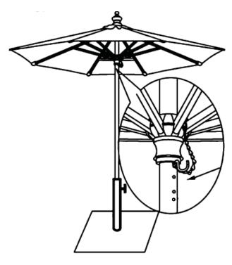
**3.** Open the umbrella by pulling down on the rope. Once the canopy is opened to the desired height secure the canopy by inserting the safety pin into the hole on the upper pole. Once the pin is in place, gently release the rope pulley. You are now ready to enjoy your wood umbrella.
